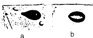
FIG. 7. Microphotographs of track of a lithium ion from opposite sides of a detector film (PAGC) through which the particle passed: a) the direction of advance of the etching is the same as the direction of motion of the ion; b) opposite directions.
